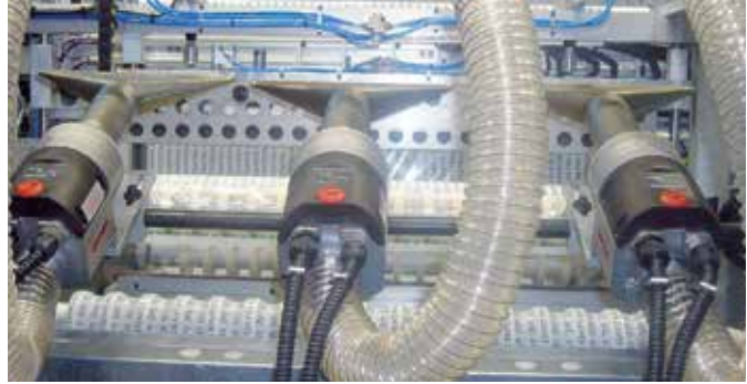
Three LHS 61S air heaters with wide slot nozzles in a wrapping line.
